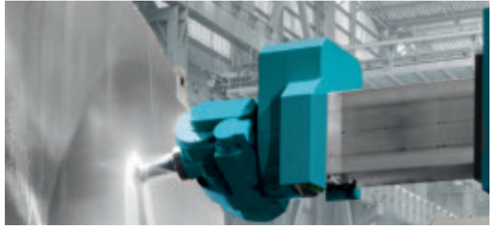
TW 2 AC 2 axes contouring head
