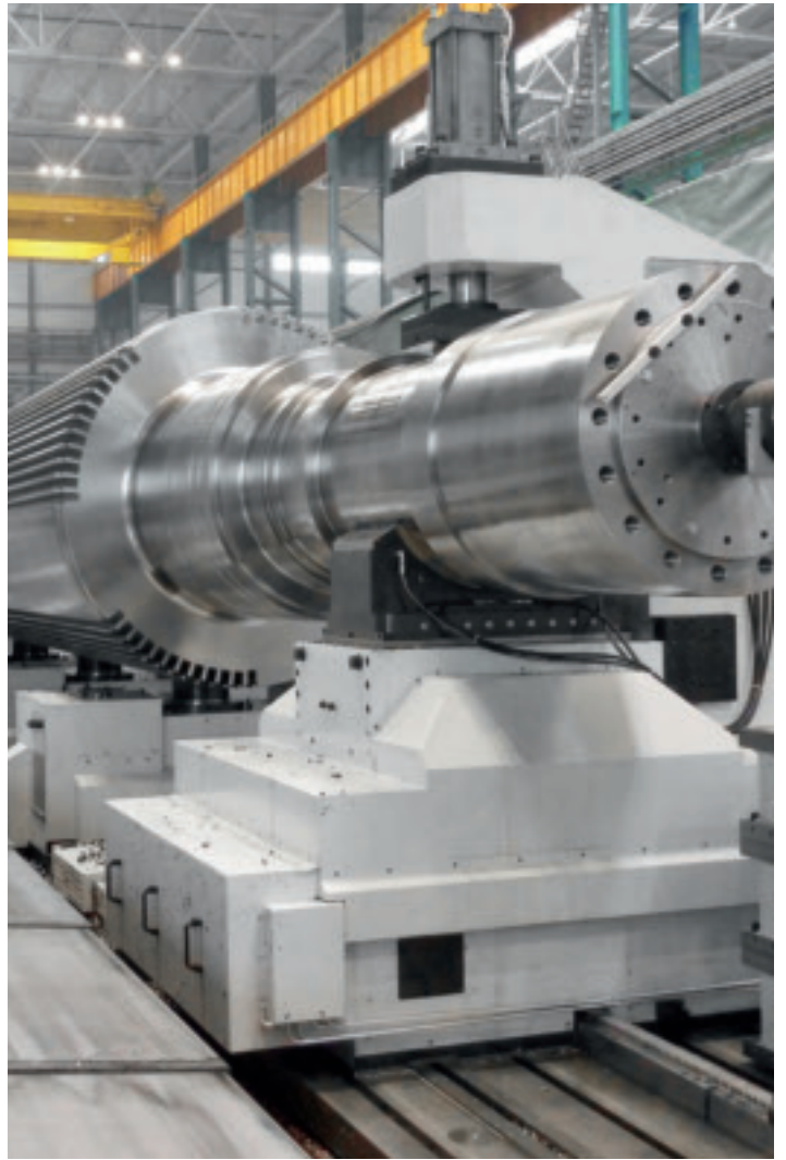
hydrostatic steady rest
