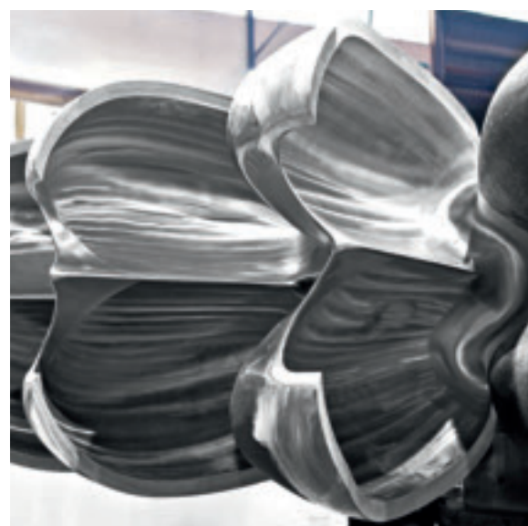
POWER GENERATION hydraulic turbine pelton rotor
