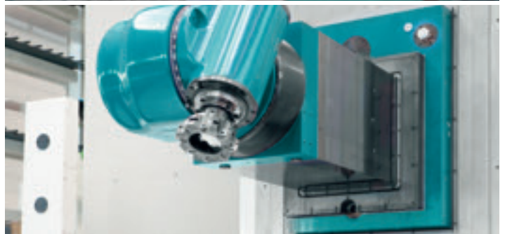
TTL universal head with orthogonal axes
