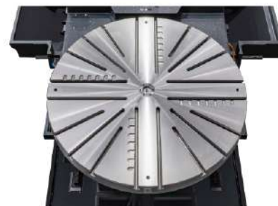
Compound T-slot (Mill-Turning, OPT.)
