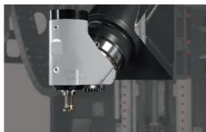
5-face machining completed chamber in one set up.
