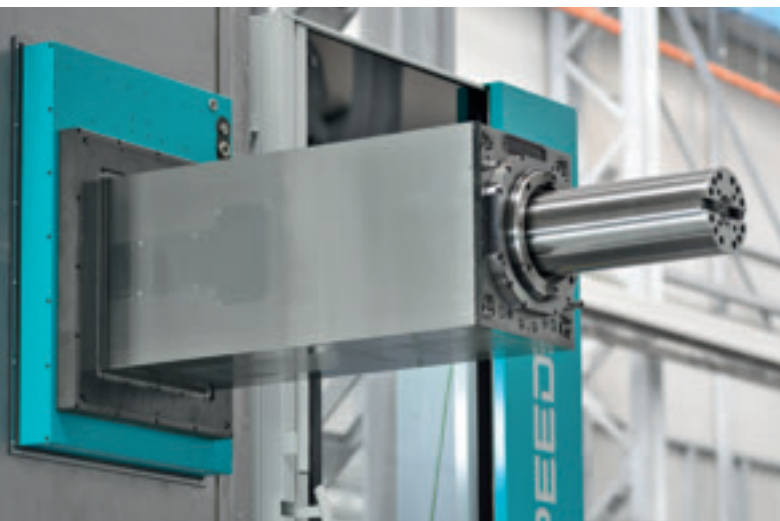
rectangular ram fully enclosed in a monolithic headstock casting with hydrostatic support on all sides
