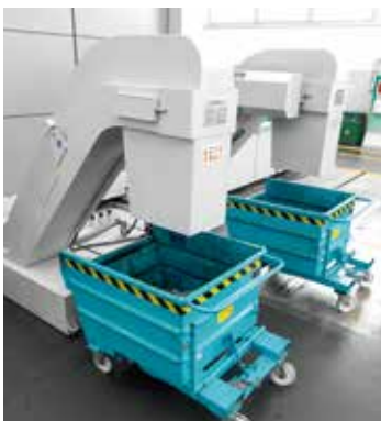
chip and coolant recovery with double chip conveyor
