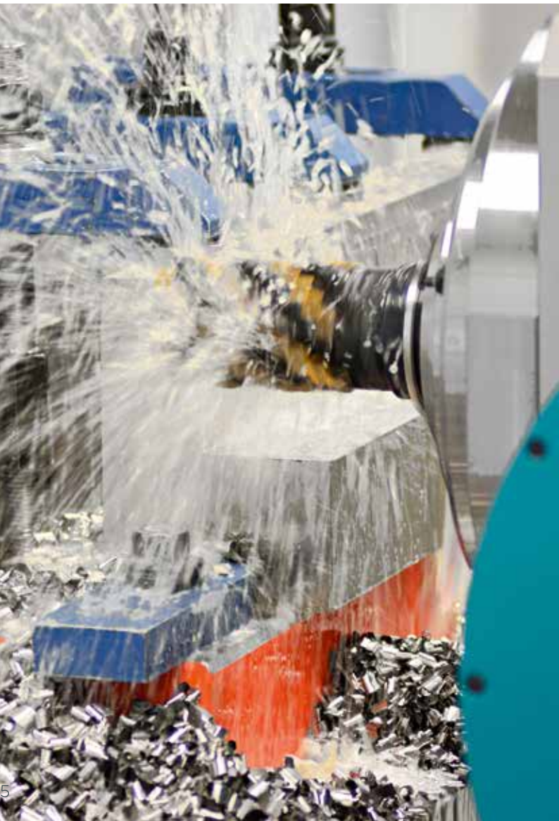
Titanium alloy machining: Ti-6AL-4V material removal rate > 500 cm 3 /min with standard headstock “AHD” in real production
