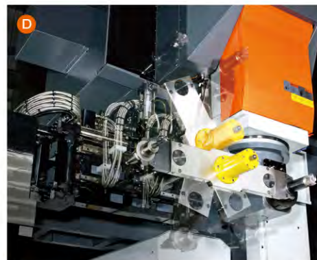
C Auto vertical-horizontal type tool magazine for vertical spindle.
