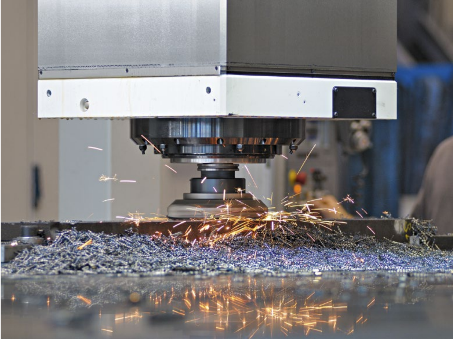
Vertiram 3000 with AL200 head heavy feed milling: material: forged steel 40CrNiMo8-6-1 milling cutter: 200 mm diameter cutting: S318 rpm - 5500 mm/min feed cutting: 2.5 mm depth, 160 mm width
