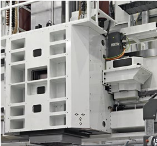
Y Axis with double preloaded pinions (VR3000-VR4000)
