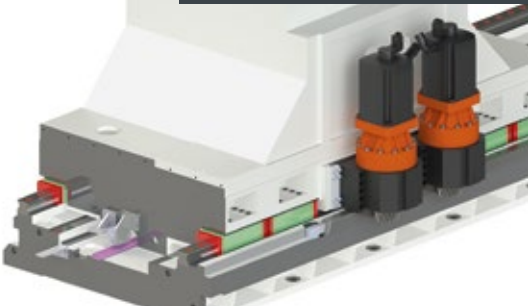
X axis with dual drive transmission (VR1000-VR2000 GT)
