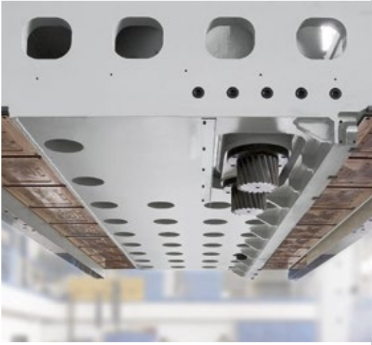
X Axis with double preloaded pinions (VR3000-VR4000 GT)
