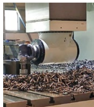
Vertiram 3000 with TS80 angle head heavy duty milling: material: forged steel 40CrNiMo8-6-1 milling cutter: 200 mm diameter cutting: S161 rpm - 707 mm/min feed cutting: 11 mm depth, 200 mm width
