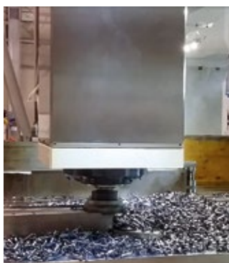
Vertiram 3000 with AL200 head heavy duty milling: material: forged steel 40CrNiMo8-6-1 milling cutter: 200 mm diameter cutting: S167 rpm - 603 mm/min feed cutting: 12 mm depth, 200 mm width
