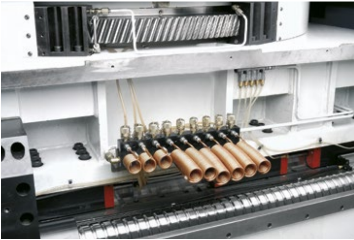
fully hydrostatic contouring table driven by a bull gear and double pinion system (preloaded for backlash free operation)
