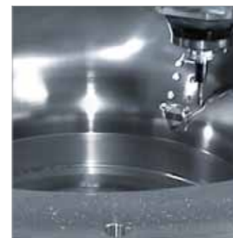
The finisher 21 kW / 130 Nm / 18.000 rpm
