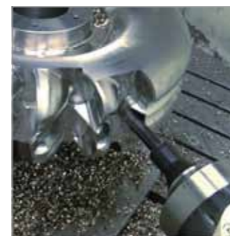
The rough cutter 34 kW / 220 Nm / 12.000 rpm
