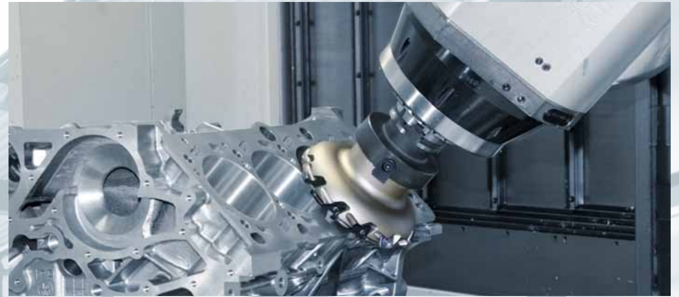
Automotive technology: motor block V8, finishing with cutter head \varnothing 100 mm
