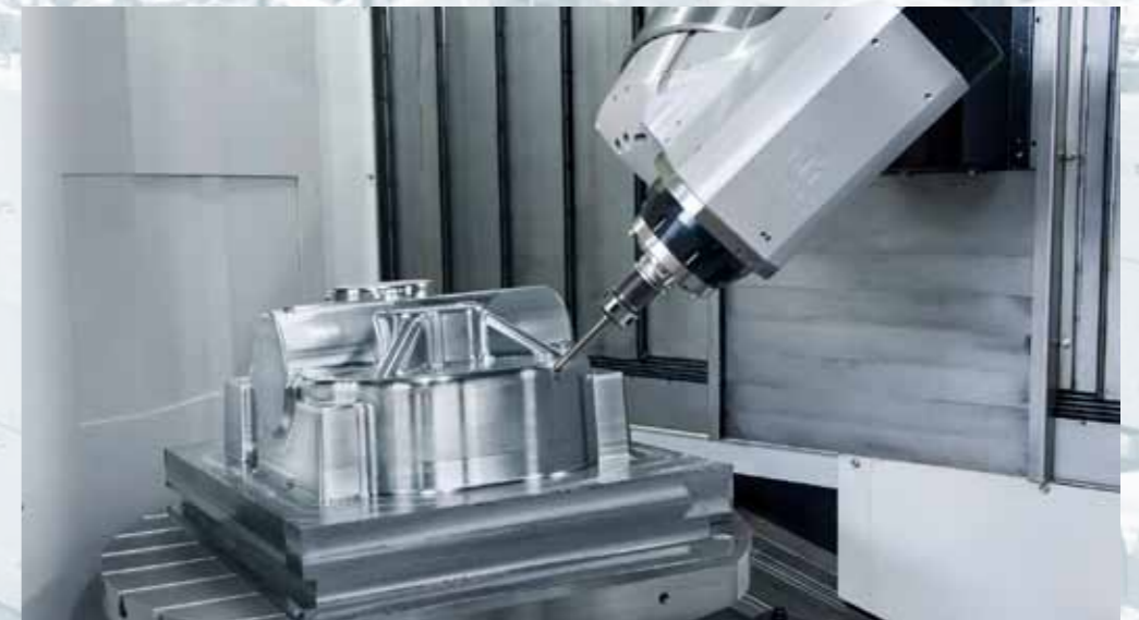
Mechanical part Ck45, 700 cm 3 /min, 170 Nm/27 kW
