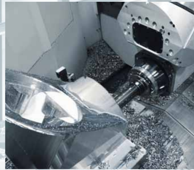
Mechanical part Ck45, 700 cm 3 /min, 170 Nm/27 kW
