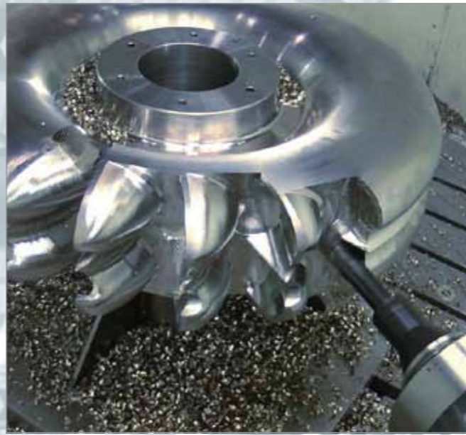
Pelton wheel 1.4313 forged, preroughing 170 Nm
