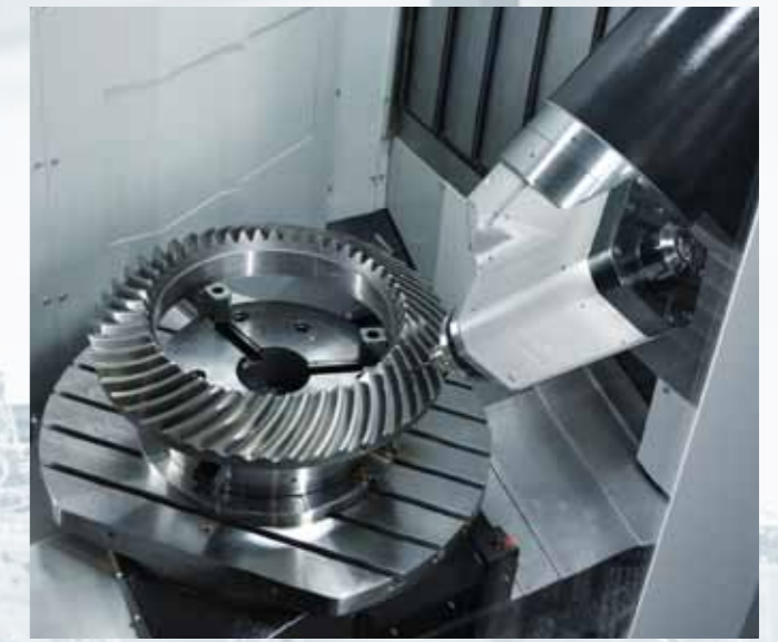
Geared rim, hard machining 12.000 rpm
