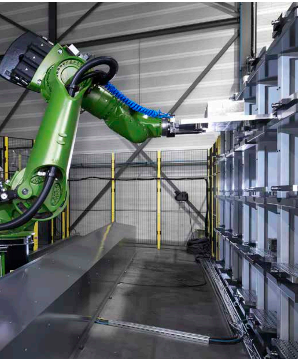
Automatic loading via pallet system
