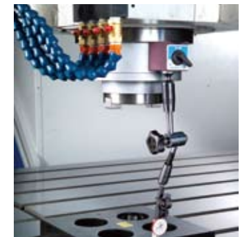
c. Geometric accuracy inspection ISO 10791-2
