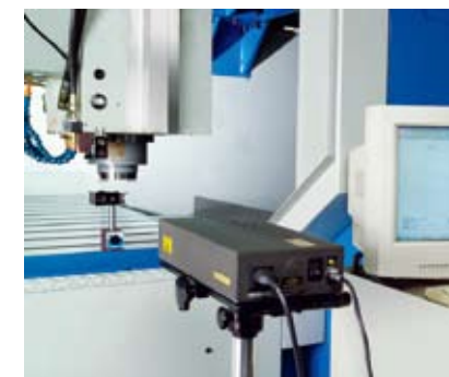
d. Positioning accuracy inspection ISO 10791-4
