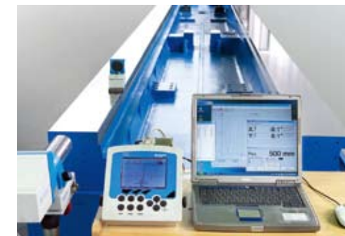
b. Laser Alignment inspection
