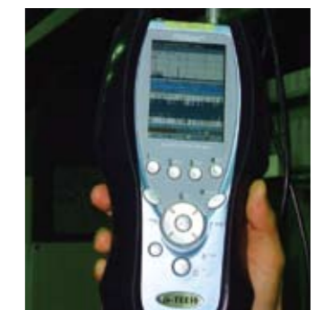
i. Noise and vibration test ISO-230
