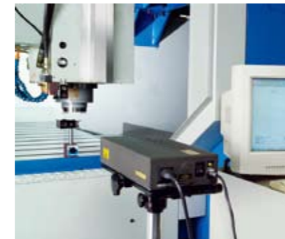
d. Positioning accuracy inspection ISO 10791-4
