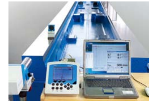
b. Laser Alignment inspection
