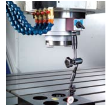
c. Geometric accuracy inspection ISO 10791-2
